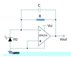
$$V_{out}(V) = I_{ph}(A) \times R(\Omega)$$
